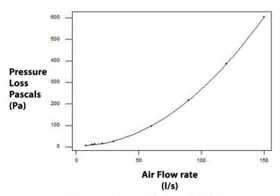
\*Pressure losses with Control Disk 10mm open
