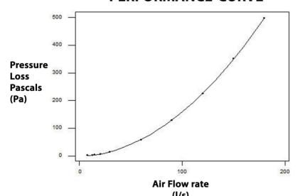
\*Pressure losses with Control Disc 10mm open
