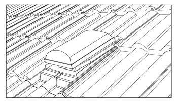
SUITABLE FOR ROOF PITCHES OF BETWEEN 20° AND 60° - FOR PITCHES ABOVE OR BELOW THIS CONSULT VORTICE TECHNICAL SERVICES
