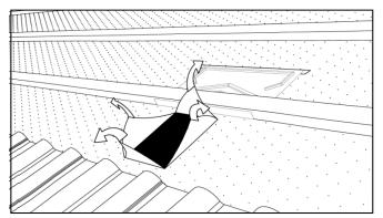
3. Lay the next course of tiles, overlapping the Universal Tile Vent Terminal on each side and compressing the foam filler. It may be necessary to remove adjacent tile nibs to prevent tiles "kicking-up". Fix adjacent tiles where necessary.
