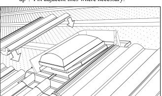
**2.** Fit the Universal Tile Vent Terminal in position and nail to the batten.
